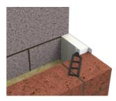
ARC Brick Ties are then used to build the closer in as the external brickwork progresses.
