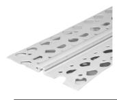
PVC Movement Beads are used to accommodate movement in plaster, stucco, or render finishes. It helps prevent cracking in large or long sections of walls or ceilings by allowing for controlled expansion and contraction.
