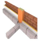
ARC's Party Wall Cavity Stop Sock is designed for use at the party wall junction; fitted in the external wall cavity, with a minimum 50mm overlap either side of the party wall cavity.
