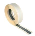
Gyproc Metal Corner Tape is a high quality paper joint tape strengthened with two corrosion-resistant galvanized steel strips for the finishing of internal and external angles in drywall construction.
